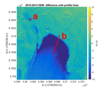
**Figure 11.** DEM difference map of the tongue of the glacier between 2010 and 2015. In red are the two lines from which profiles were extracted: "a" for the ice-cored moraine and "b" for the glacier terminus.
