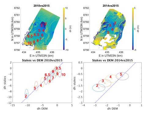
**Figure 13.** Top: position of mass balance stakes overlayed on the DEM difference for 2010–2015 (left) and 2014–2015 (right). Bottom: height variation at the stake positions according to the DEMs (x axis) versus according to the stake measurements (y axis).
