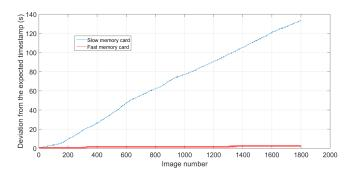
**Figure 3.** Differences between expected time stamps of pictures for a 30 min period with a lapse time of 1 s and the EXIF time stamp recovered from the first 1800 images of a GoProH3+BE. Results are either for a relatively slow micro-SD card (64 GB SanDisk Ultra microSDXC Class 10 UHS-I) or a fast card (32 GB SanDisk Extrem Plus microSDHC UHS-I/U3). The fast card diverges by only 2 s after 30 min, while the slow card diverges by 134 s at a visibly irregular rate.
