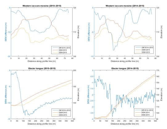
**Figure 12.** Profiles extracted from the 2010, 2014, and 2015 DEMs, and DEM differences associated with them. Top is profile "a" from Fig. 11 and bottom is profile "b". Blue lines are DEM differences (scale on the left axis) while red and orange are the DEM values (scale on the right axis; red is the older of the two DEMs).
