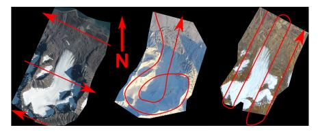
Figure 9. Orthoimages produced for the UltraCam data of 2010 (left), GoPro 2014 (middle), and GoPro 2015 (right). Flight lines are indicated in red.
