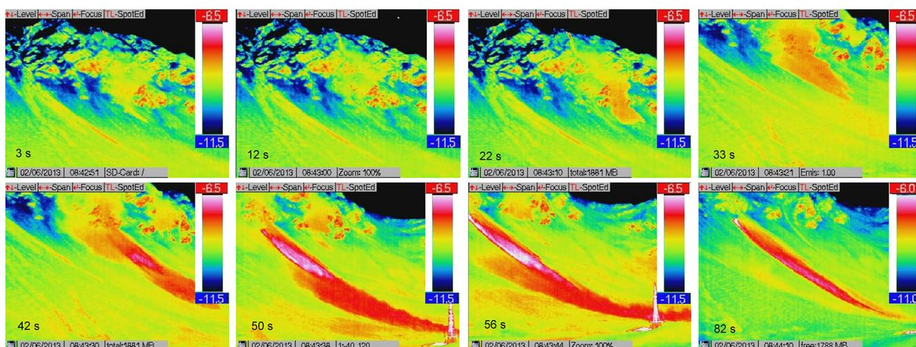
**Figure 5.** Screenshot of IRT camera videos for avalanche #2. The first picture was taken 3 s after the avalanche released. Note that the temperature scale was changed by 0.5 °C for the last shown image (82 s).
